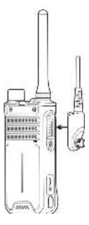
3. Tighten the screw on the audio accessory plug.
