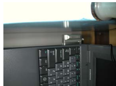
Figure 26. Body SAR Test Setup
