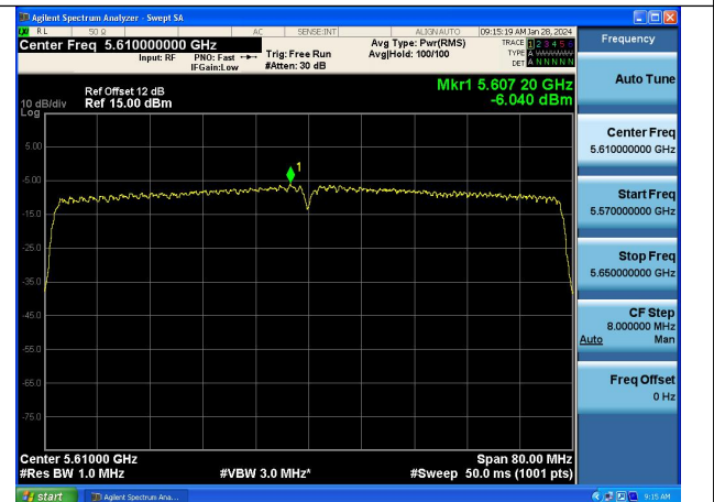
Mode:802.11ac VHT80 Frequency:5610MHz Ant:Chain1
