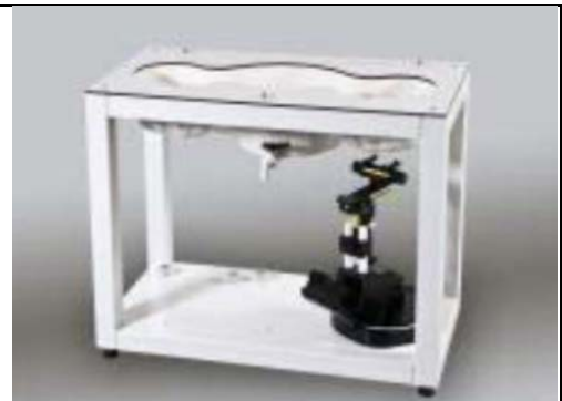
Fig. 6.8 Photo of SAM Phantom
