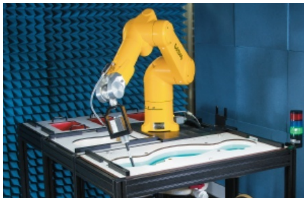
Fig 6.5 Photo of DASY5
