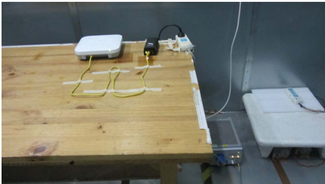
Picture 3 Conducted Emission Test Setup
