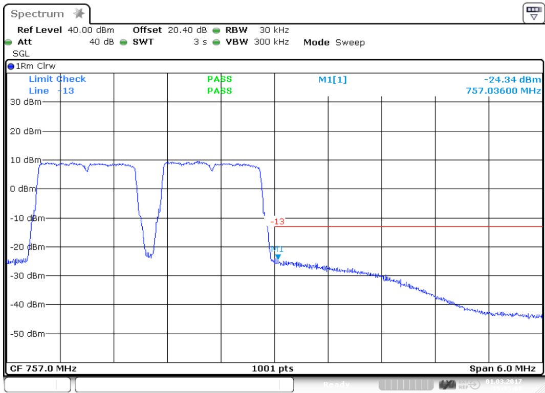
plot 8.3.2.2-#1 Intermodulation: §27.53, §2.1051; Test results; Downlink LTE 746 – 757MHz Lower Band Edge
