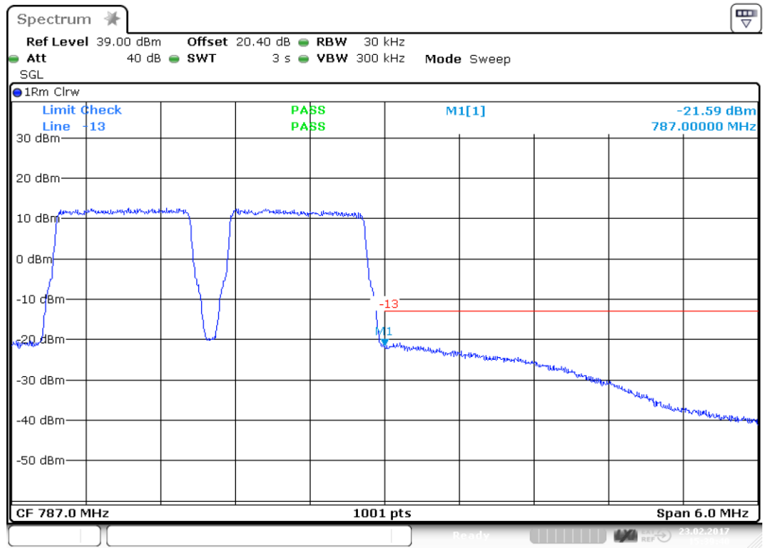
plot 8.3.2.4-#1 Intermodulation: §27.53, §2.1051; Test results; Uplink LTE 776 – 787MHz Lower Band Edge
