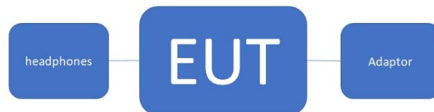
Fig. 2-3 Conducted (AC powerline) Emission Configuration
