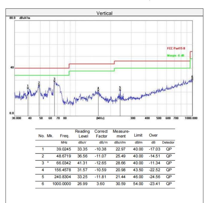
Final Level =Receiver Read level + Correct Factor
