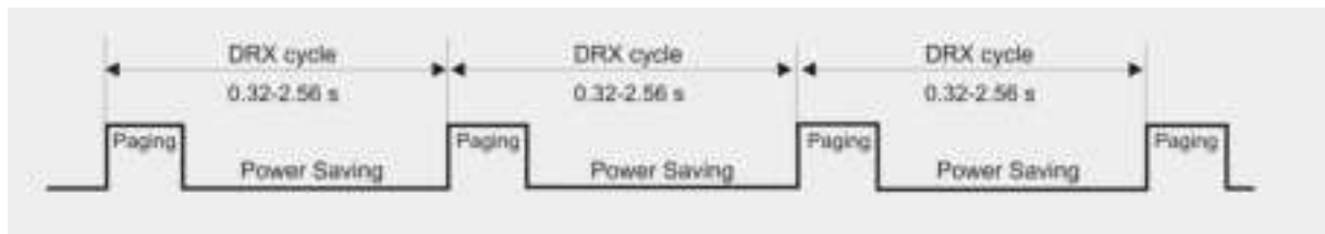
Figure 38: Power saving and paging in LTE networks
