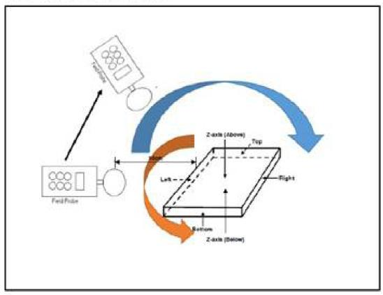
Note: Measurements were made from all sides and the top of the primary/client pair, with the 15/20cm measured from the center of the probe(s) to the edge of the device.
