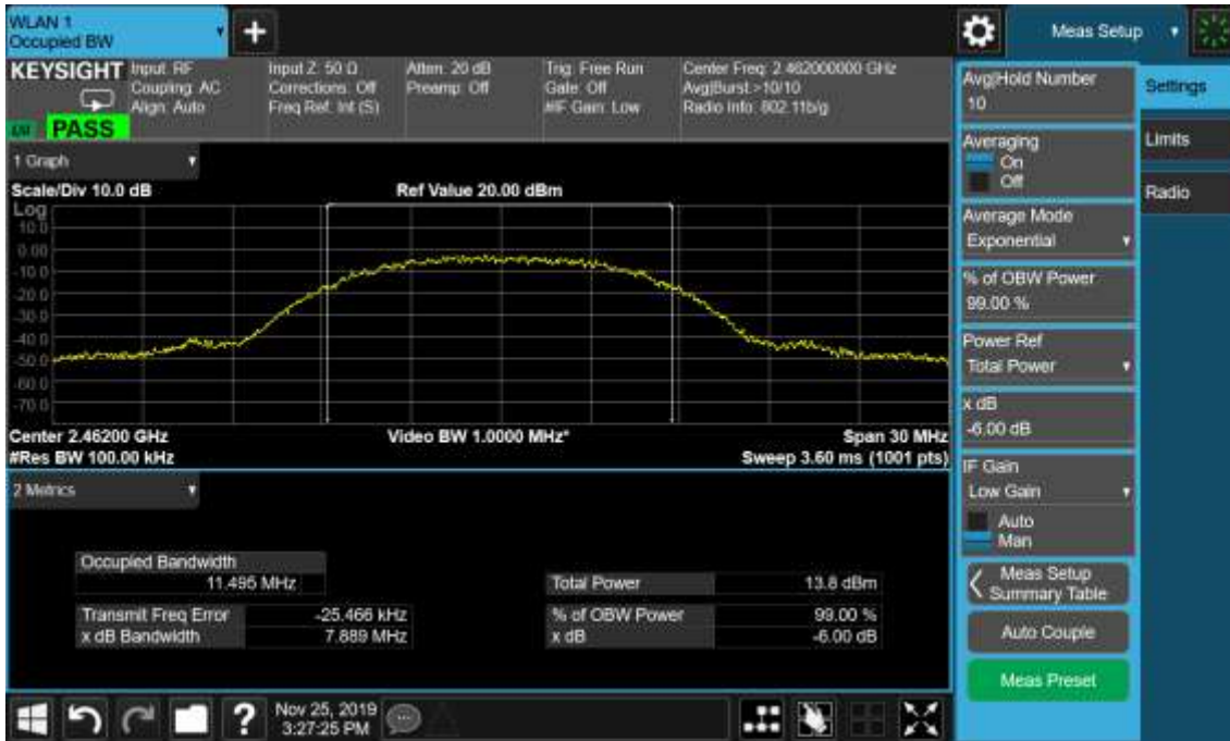
Figure 3: 6dB Bandwidth and 99% Bandwidth, 802.11b, 2462MHz
