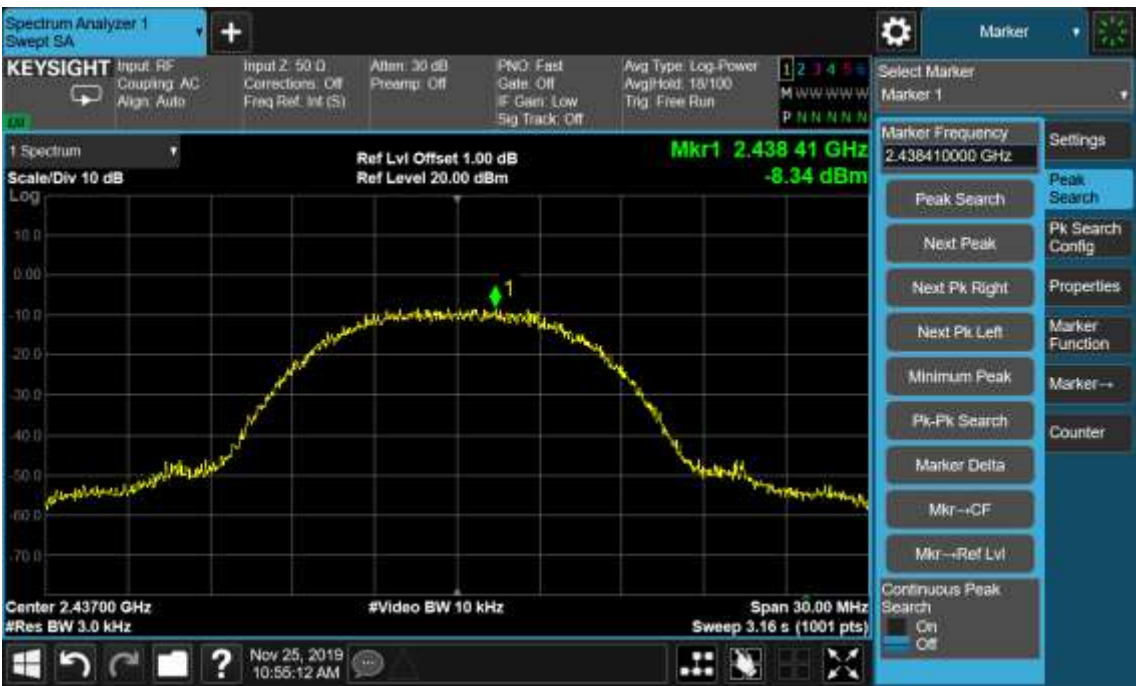
Figure 11: Power Spectral Density, 802.11b, 2437MHz
