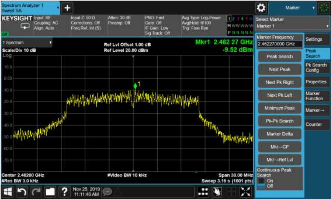
Figure 15: Power Spectral Density, 802.11g, 2462MHz
