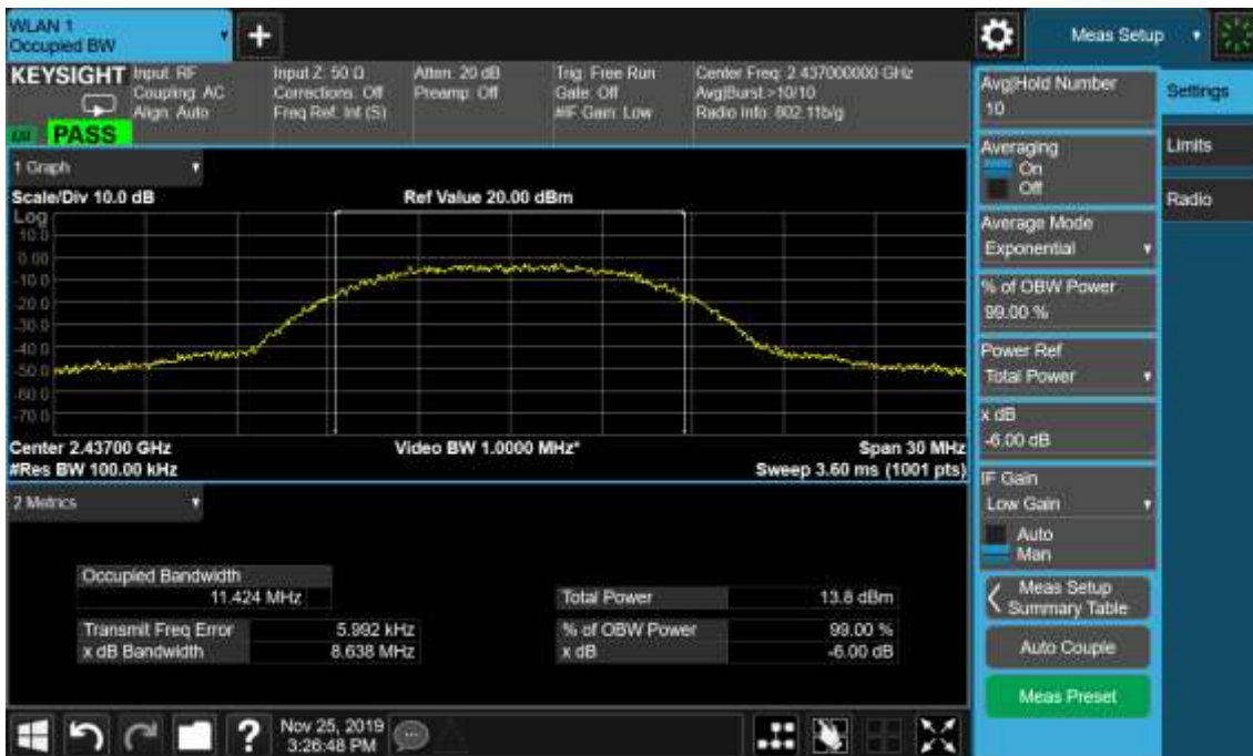
Figure 2: 6dB Bandwidth and 99% Bandwidth, 802.11b, 2437MHz
