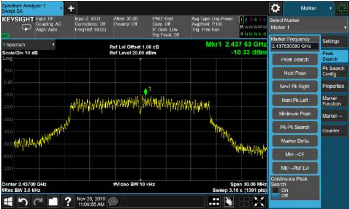
Figure 14: Power Spectral Density, 802.11g, 2437MHz
