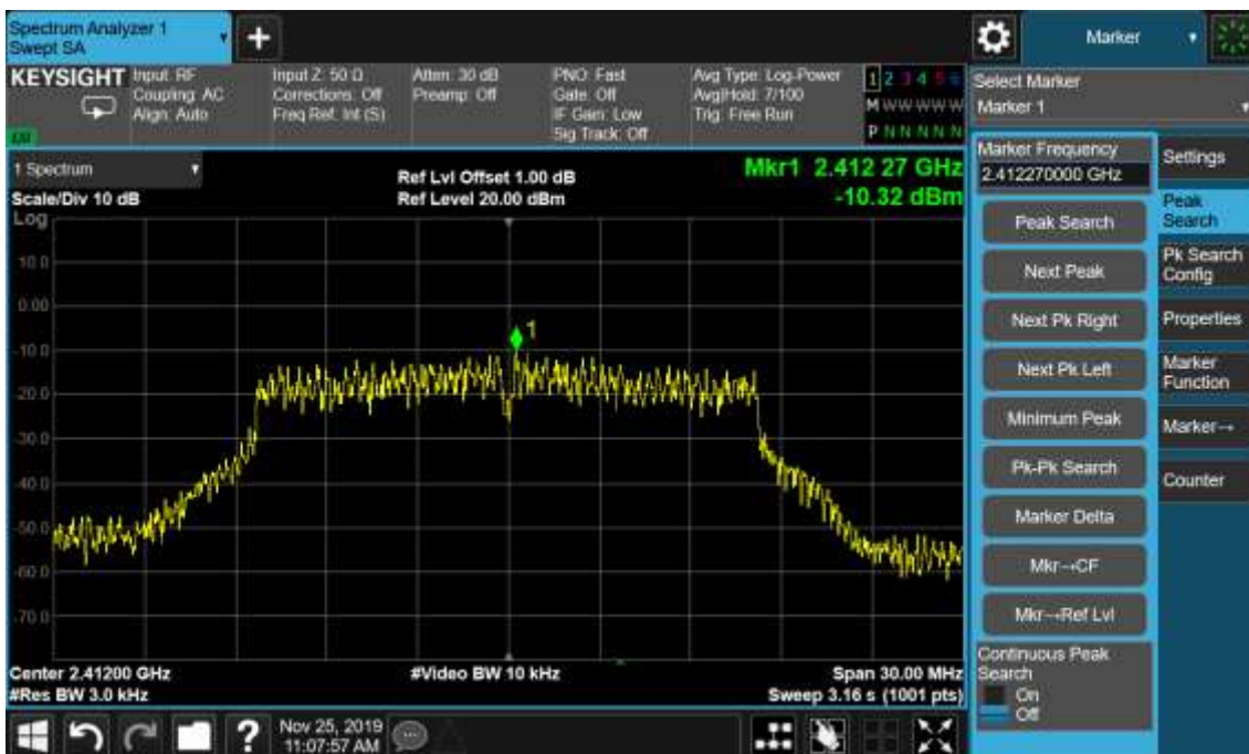
Figure 13: Power Spectral Density, 802.11g, 2412MHz
