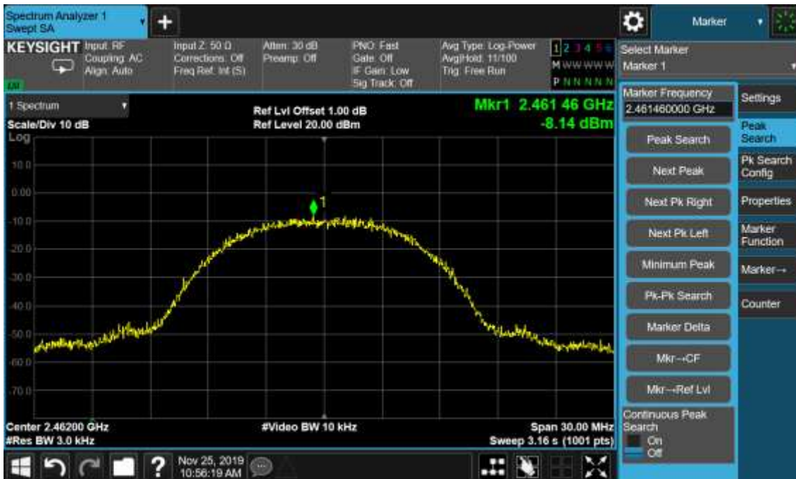
Figure 12: Power Spectral Density, 802.11b, 2462MHz
