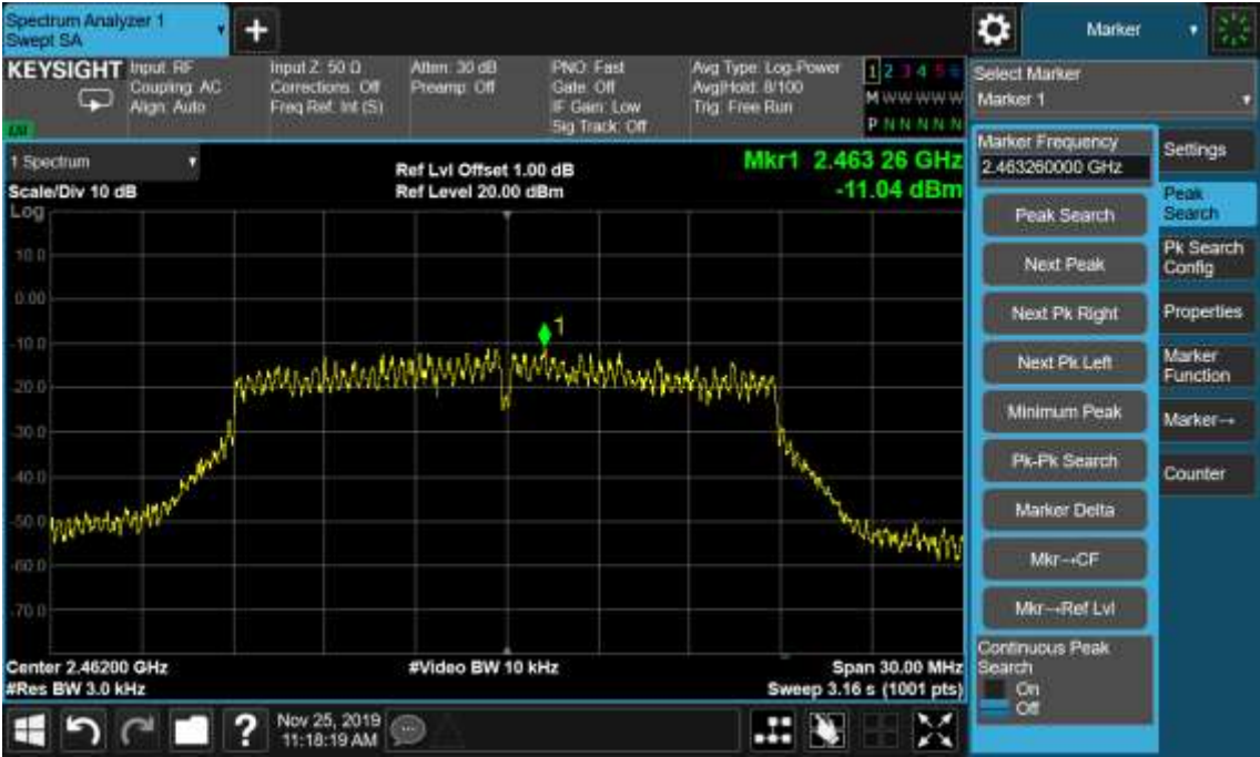
Figure 18: Power Spectral Density, 802.11n(HT20), 2462MHz
