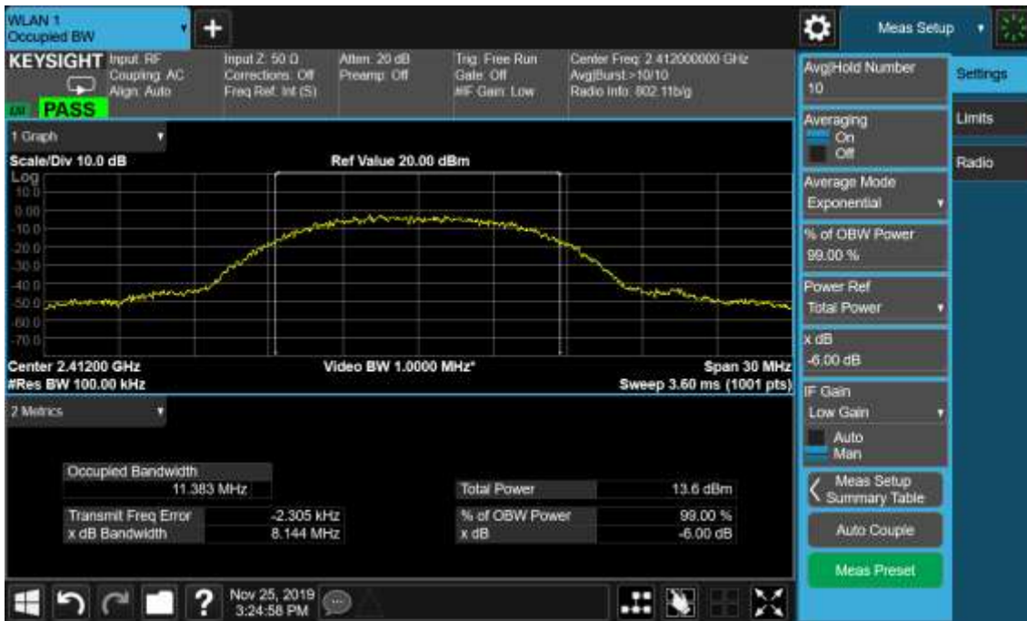
Figure 1: 6dB Bandwidth and 99% Bandwidth, 802.11b, 2412MHz
