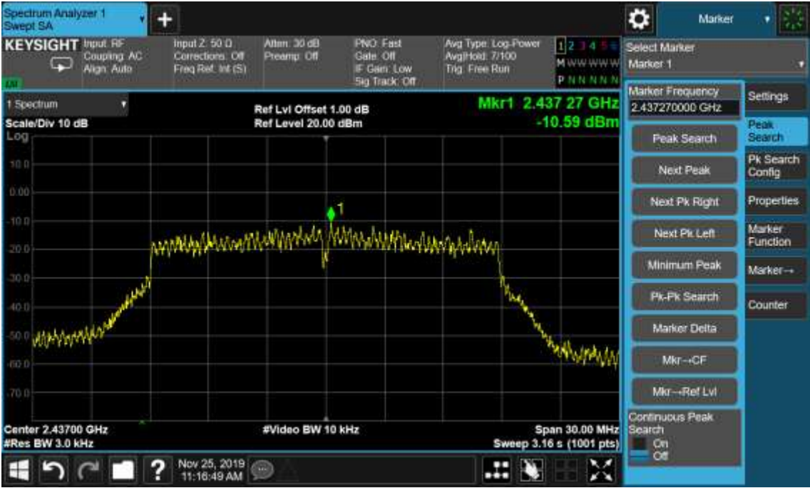
Figure 17: Power Spectral Density, 802.11n(HT20), 2437MHz
