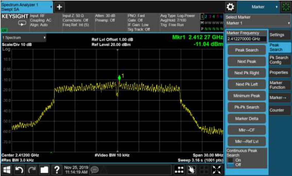
Figure 16: Power Spectral Density, 802.11n(HT20), 2412MHz
