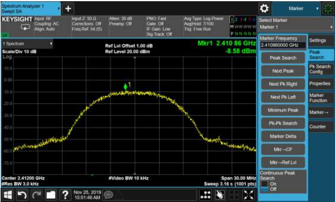
Figure 10: Power Spectral Density, 802.11b, 2412MHz
