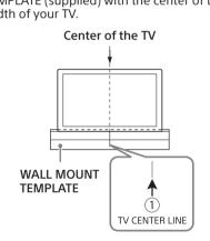
3 Align the "← ② TV BOTTOM LINE" printed on the WALL MOUNT TEMPLATE with the bottom of your TV, then adhere the WALL MOUNT TEMPLATE on the wall with a commercially
