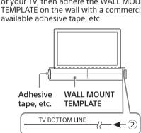
**4** Fasten the screws prepared in step 1 securely into the screw marks (®) on the "← ③ SCREW LINE" printed on the WALL MOUNT TEMPLATE
