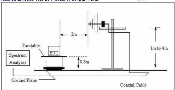
(C) Radiated Emission Test-Up Frequency Above 1GHz
