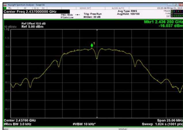
Power spectral density-802.11g ,2412MHz
