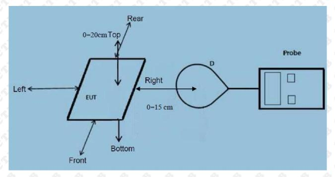
Note: Measurements should be made from all sides and the top of the primary/client pair, with the 20 cm-0cm measured from the center of the top, and 15cm-0cm measured from the center of the rest
