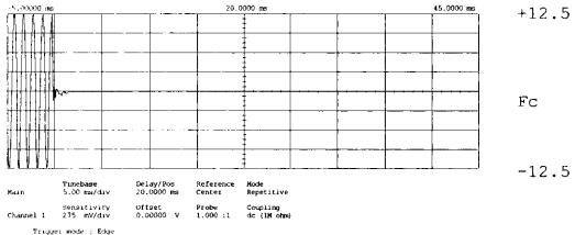
Trigger mode : Edge On Negative Edge Of Chan2 Trigger Level Chan2 = 55.500 mV (noise reject ON) Holdoff = 40.000 ms
