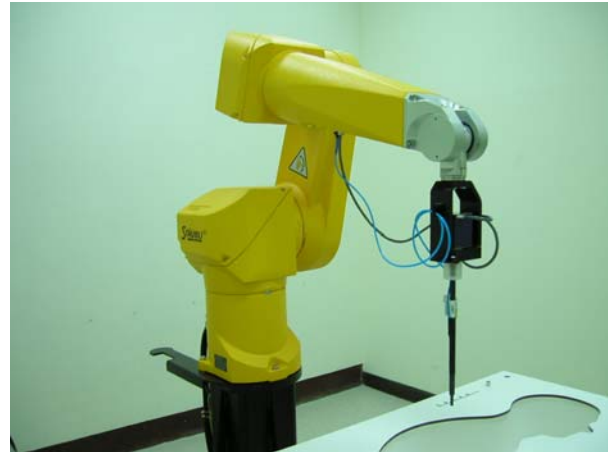
Fig. 5.2 Probe setup on robot
