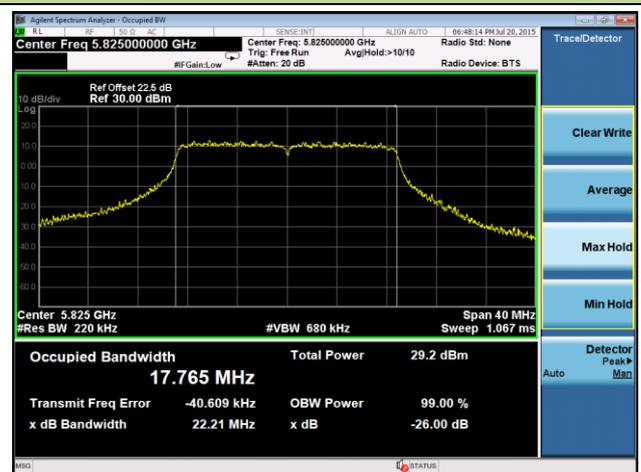
**802.11ac-VHT40 26dB Bandwidth & 99% Bandwidth - Ant 1**
