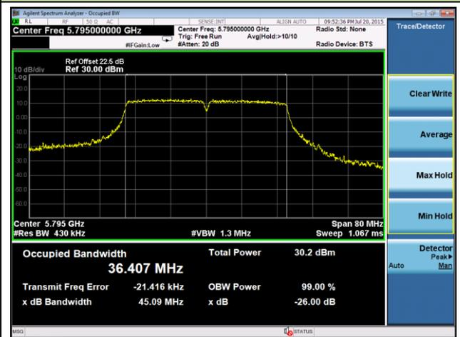
**802.11ac-VHT20 26dB Bandwidth & 99% Bandwidth - Ant 2**
