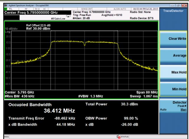
**802.11ac-VHT20 26dB Bandwidth & 99% Bandwidth - Ant 1**
