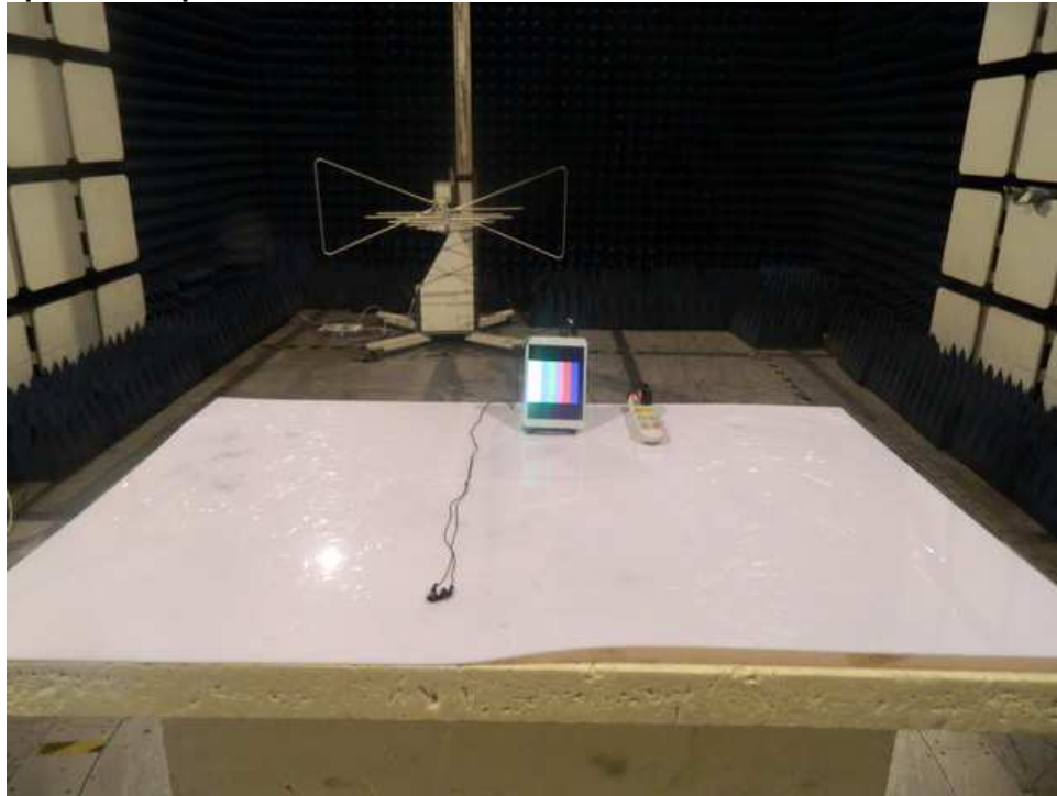
Photograph 2: Set-up for Radiated Emission of below 1GHz
