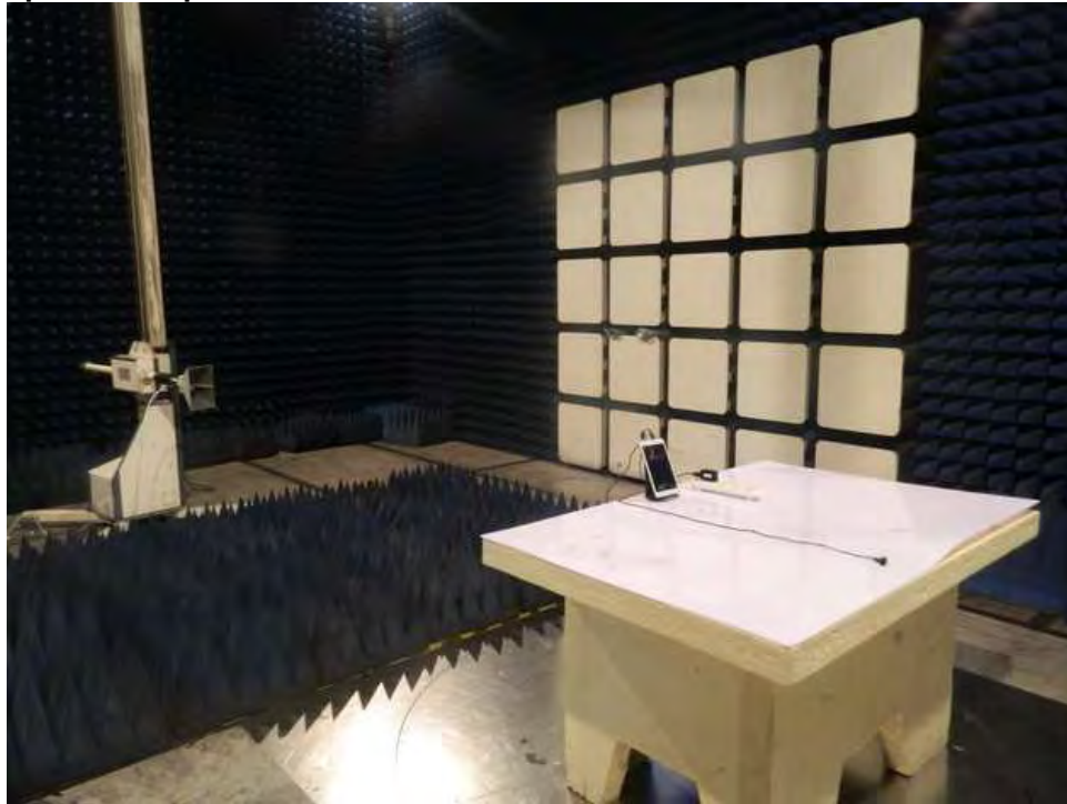
Photograph 3: Set-up for Radiated Emission of 1 - 6GHz
