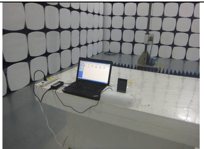
Radiated Spurious Emissions Test Setup Above 1GHz
