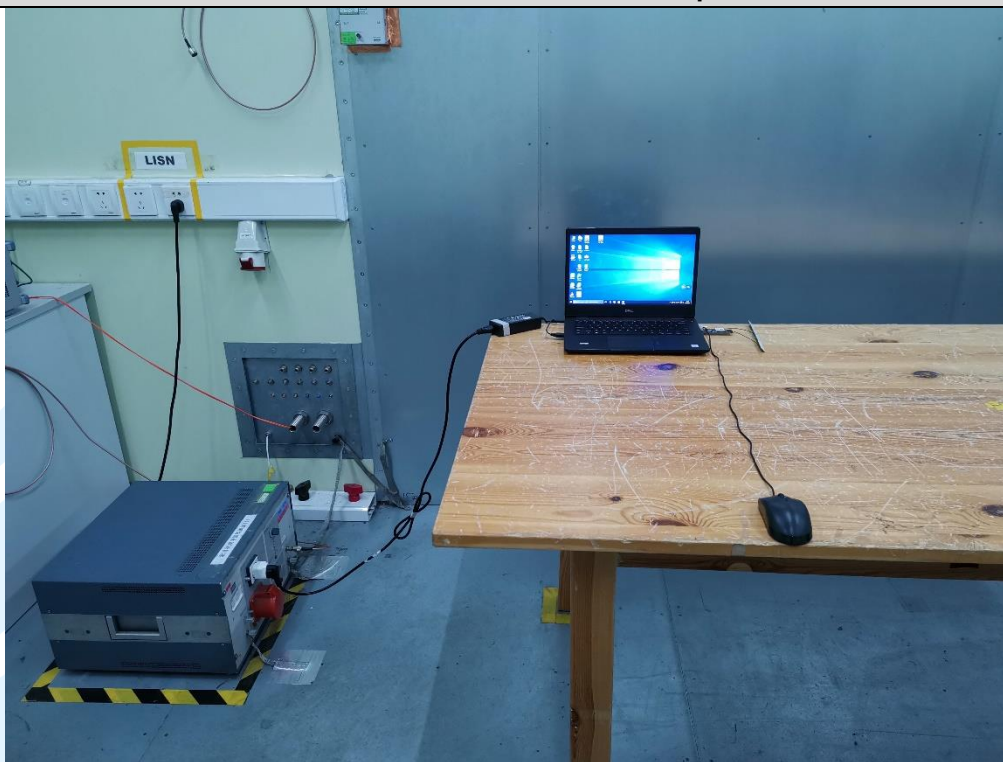
Conducted Emission Test Setup
