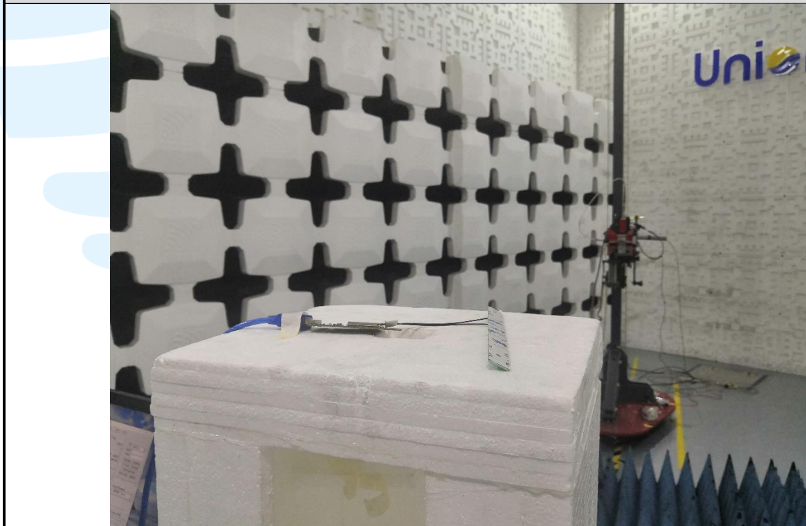
Radiated emission Test Setup (Above 1 GHz)
