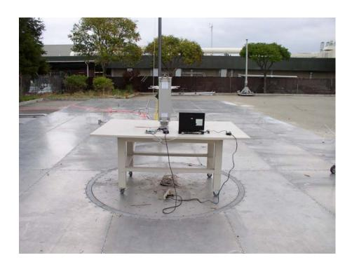
Radiated Emission, EUT (module) with Load / Notebook, CW mode
