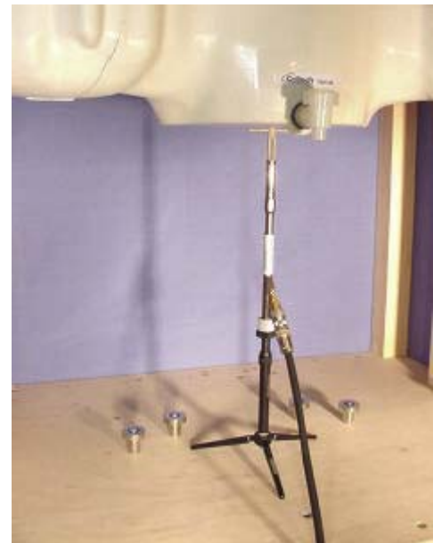
1800MHz System Check Setup
