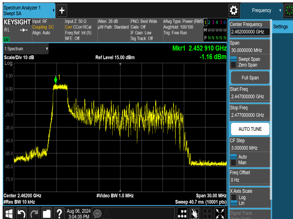
Plot 7-33. Power Spectral Density Plot SISO ANT2 (802.11ax/be OFDMA – 26 Tones – Ch. 11)
