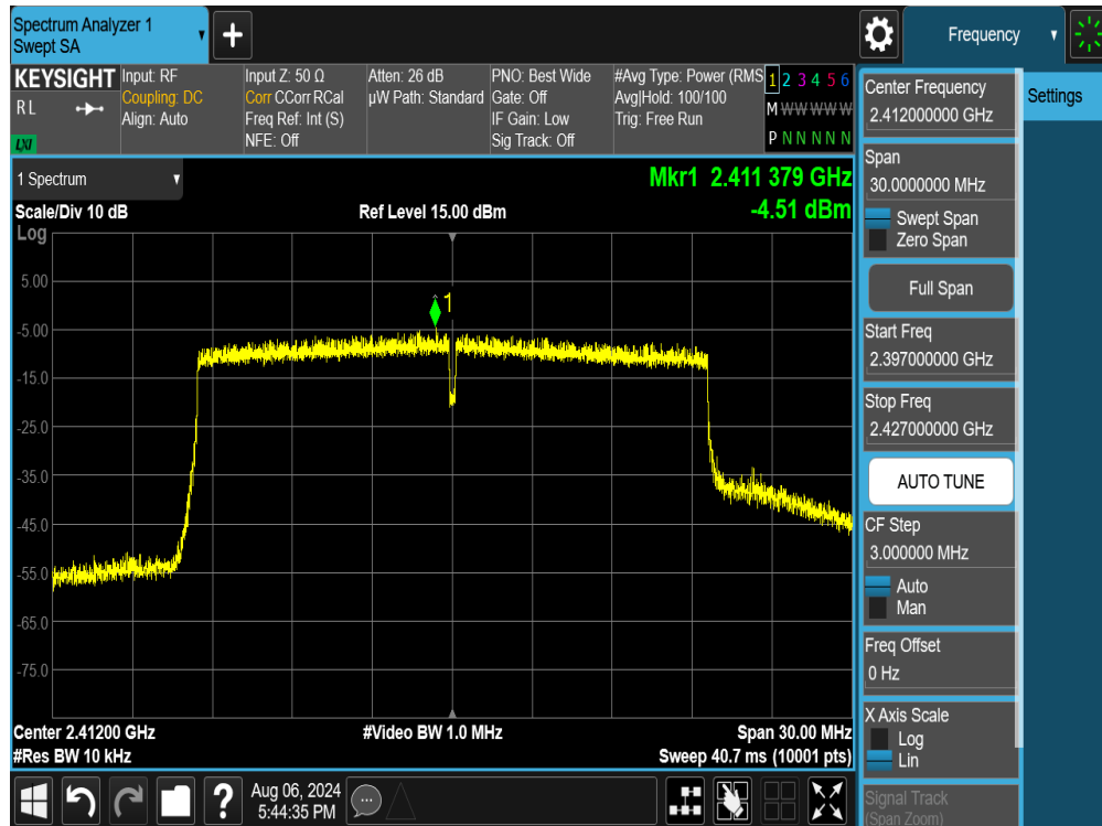
Plot 7-34. Power Spectral Density Plot SISO ANT2 (802.11ax/be OFDMA – 242 Tones – Ch. 1)
