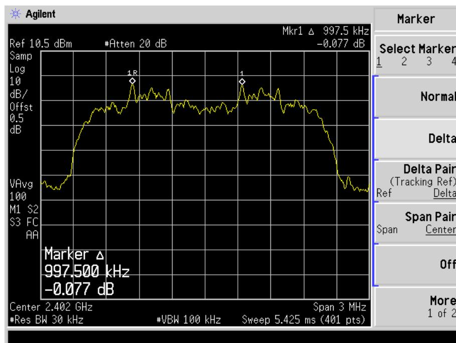
Channel Spacing (Middle CH=1MHz)
