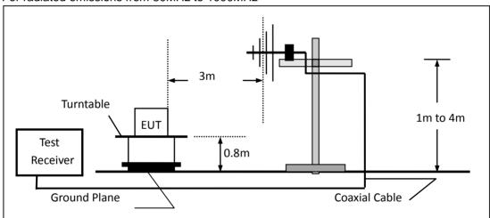
(c) For radiated emissions above 1000MHz
