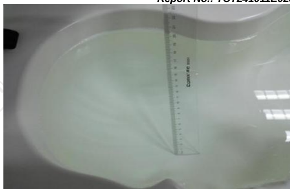
The Head Liquid of 2450MHz (15.6cm)
