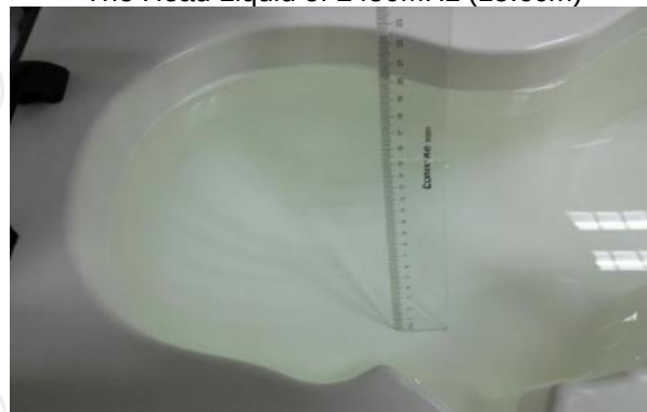
The Head Liquid of 1800MHz (15.2cm)
