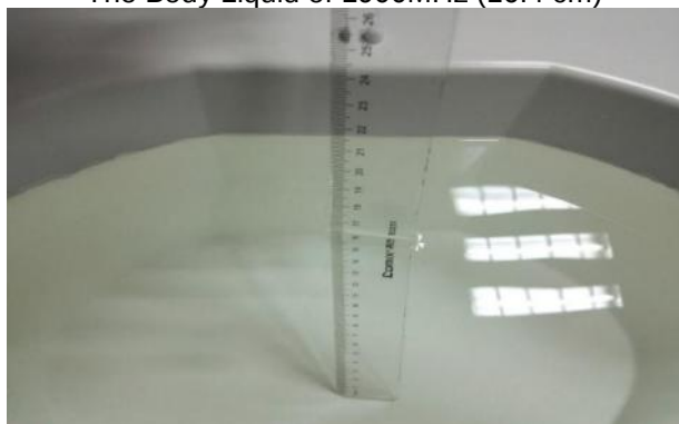
The Body Liquid of 2600MHz (16.5cm)
