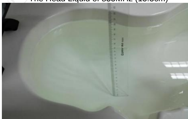
The Head Liquid of 2600MHz (15.1cm)
