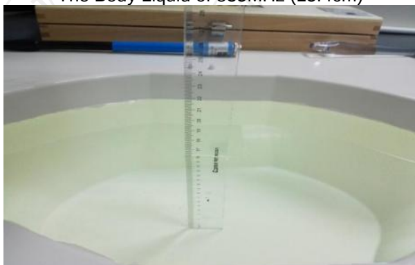
The Body Liquid of 1900MHz (16.4 cm)
