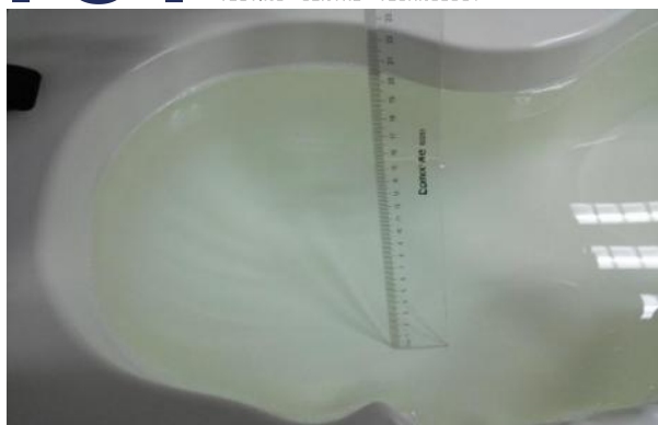
The Head Liquid of 1900MHz (15.5cm)
