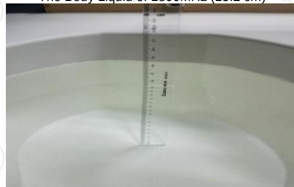
The Body Liquid of 2450MHz (15.3cm)
