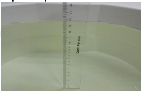
The Body Liquid of 835MHz (15.4cm)
