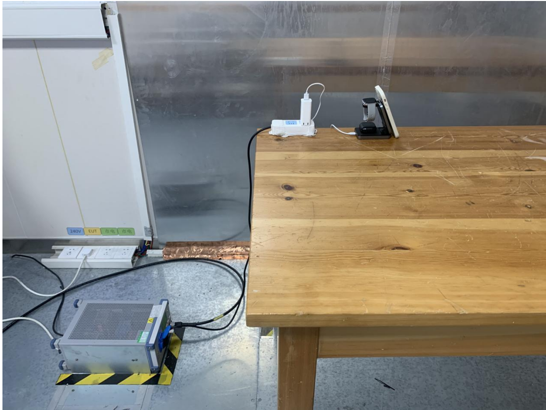
Conducted emission test setup
