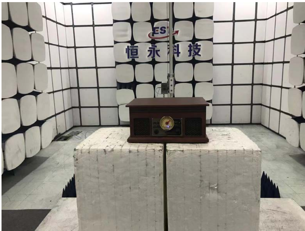
Radiated emission test: Above 1GHz
