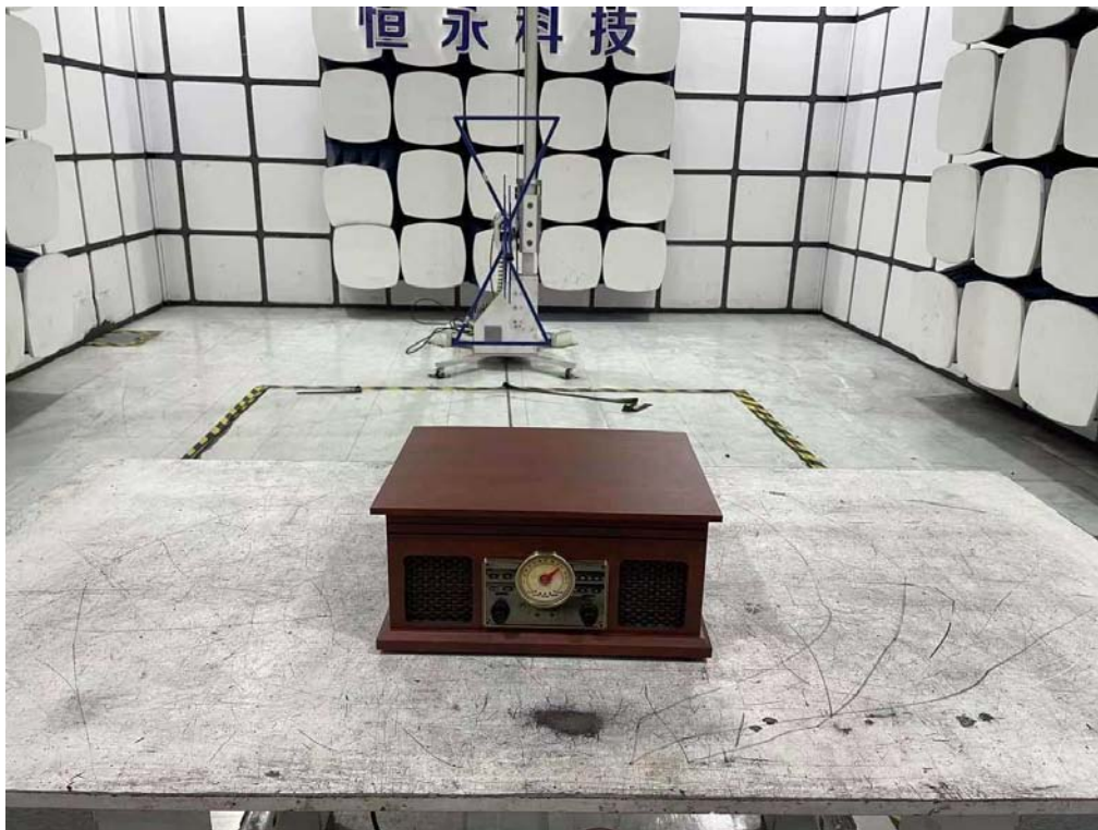
Radiated emission test: Below 1GHz
