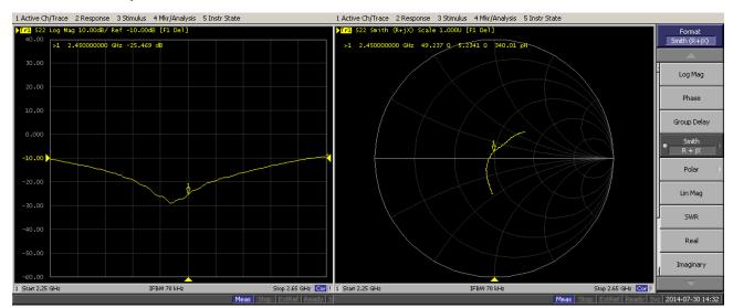
Per IEEE Std 1528-2003, the dipole should have a return loss better than -20dB at the test frequency to reduce uncertainty in the power measurement.
