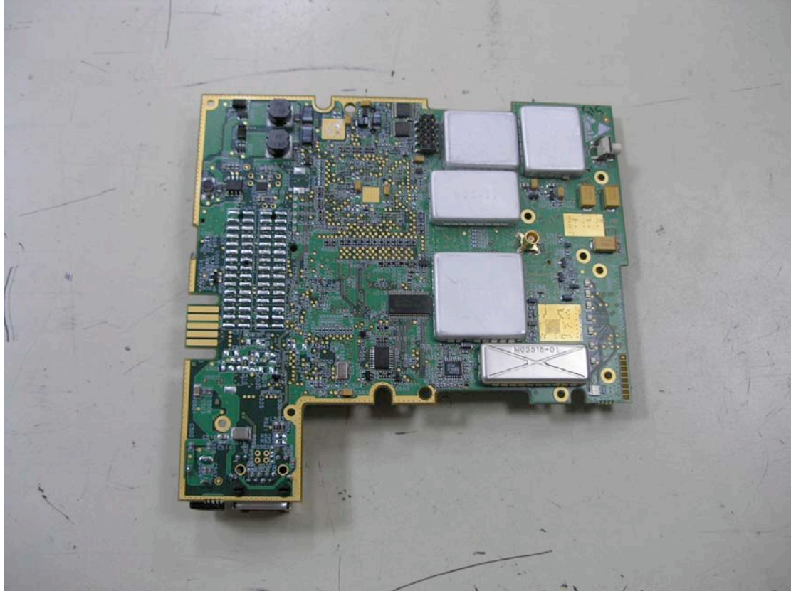
BreezeMAX 2300 CPE Si with RF covers on
