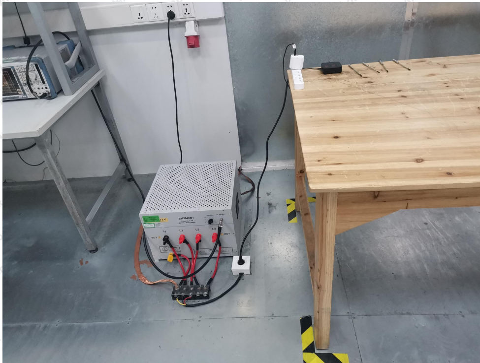
Photo of Conducted Emission Measurement
