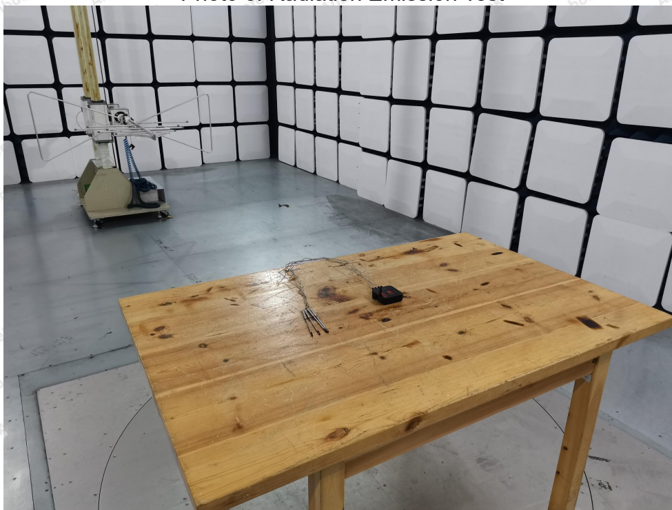
Photo of Radiation Emission Test
