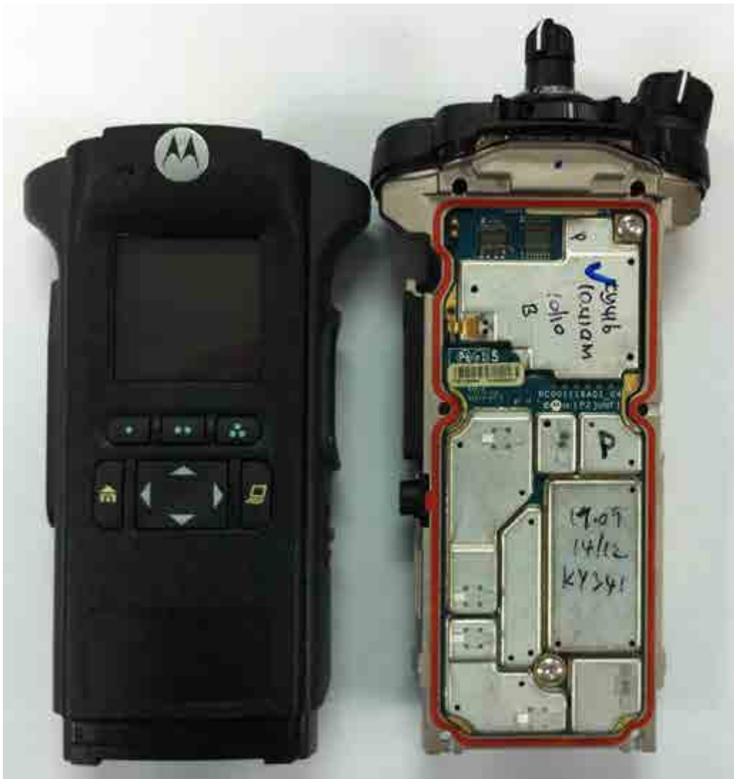
RF and Vocon boards with chassis and housing (APX6000/ APX6000Li/APX5000 Model 2.5) (Front side)
