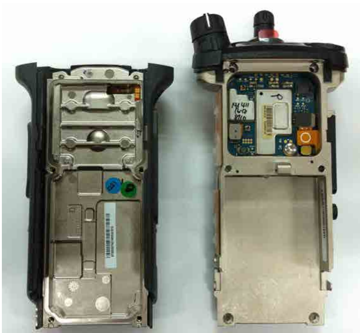
Expansion board with chassis and housing (APX6000/ APX6000Li/APX5000 Model 1.5) (Back side)
