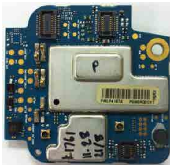
Expansion board with shields (Top) (APX6000/APX5000/APX6000XE/APX6000Li)
