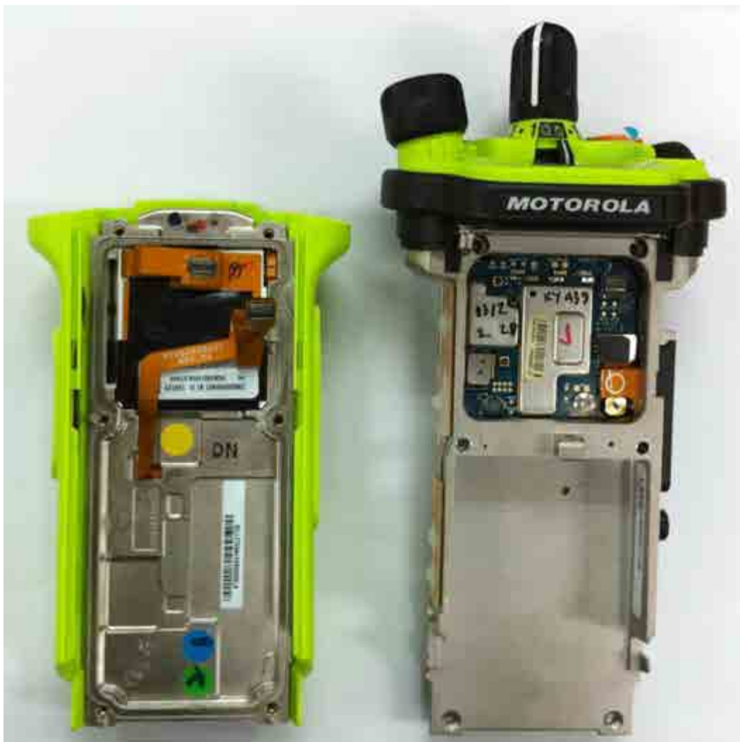
Expansion board with chassis and housing of APX6000XE Model 3.5 (Back side)
