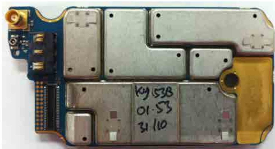
RF board with Shields (Bottom) (APX6000/APX5000/APX6000XE/APX6000Li)
