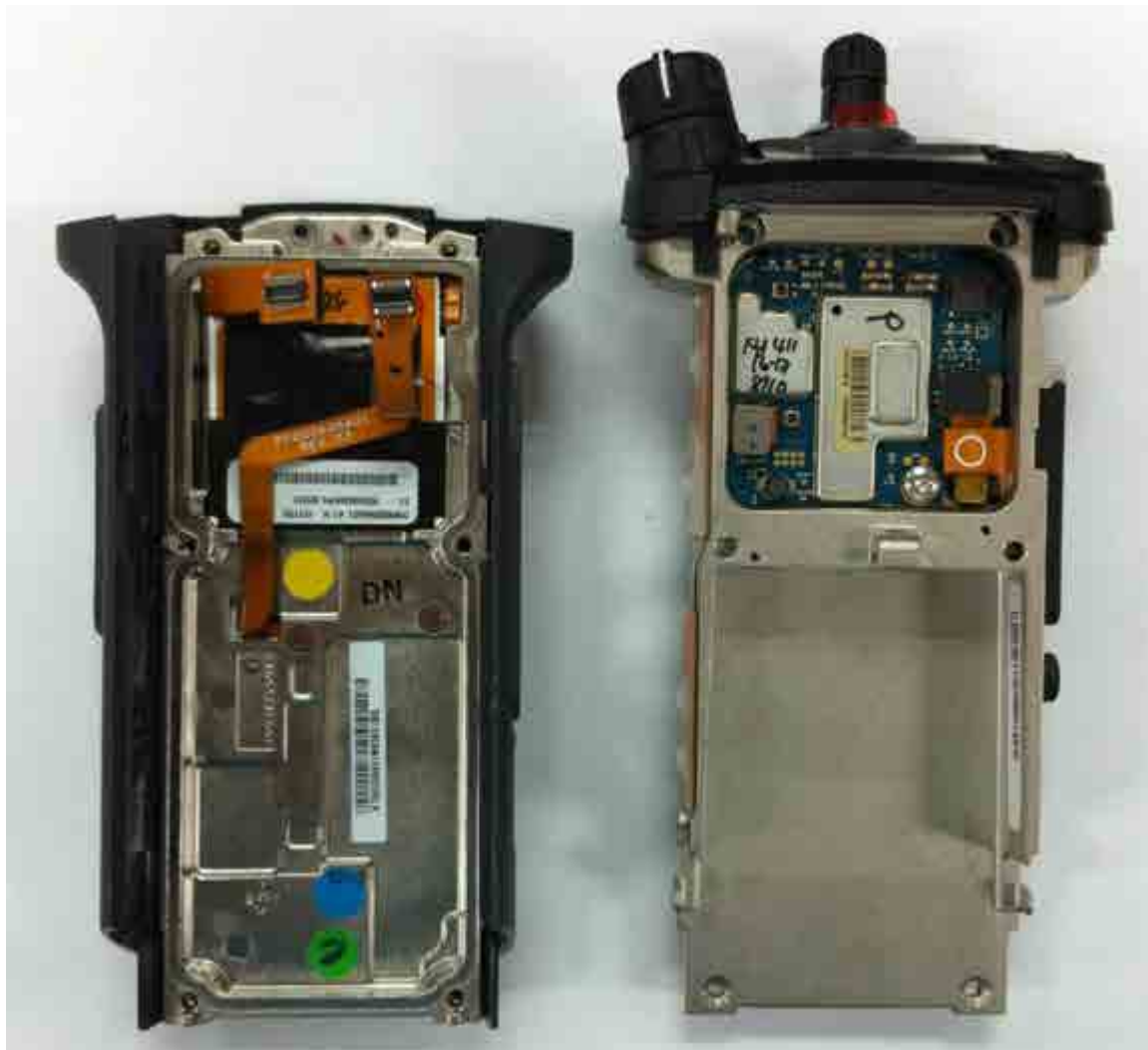
Expansion board with chassis and housing (APX6000/ APX6000Li/APX5000 Model 2.5) (Back side)
