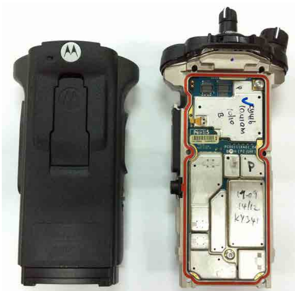
RF and Vocon boards with chassis and housing (APX6000/ APX6000Li/APX5000 Model 1.5) (Front side)
