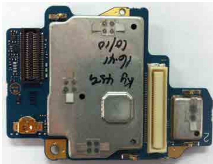
Vocon board with shields (Bottom) (APX6000/APX5000/APX6000XE/APX6000Li)
