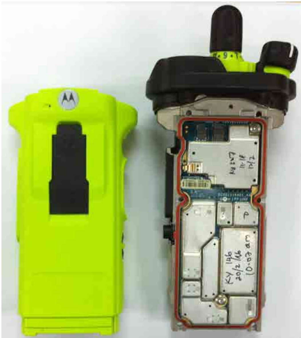
RF and Vocon boards with chassis and housing of APX6000XE Model 1.5 (Front side)
