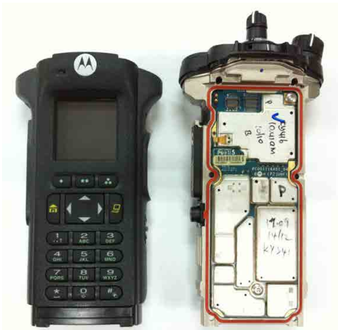
RF and Vocon boards with chassis and housing (APX6000/ APX6000Li/APX5000 Model 3.5) (Front side)
