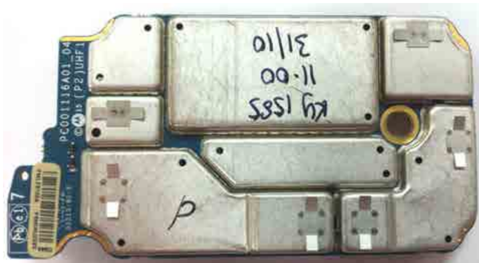
RF board with Shields (Top) (APX6000/APX5000/APX6000XE/APX6000Li)
