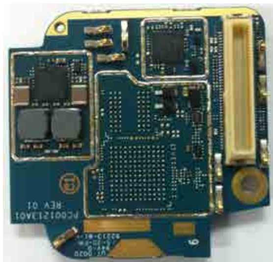
Expansion board without shields (Bottom) (APX6000/APX5000/APX6000XE/APX6000Li)
