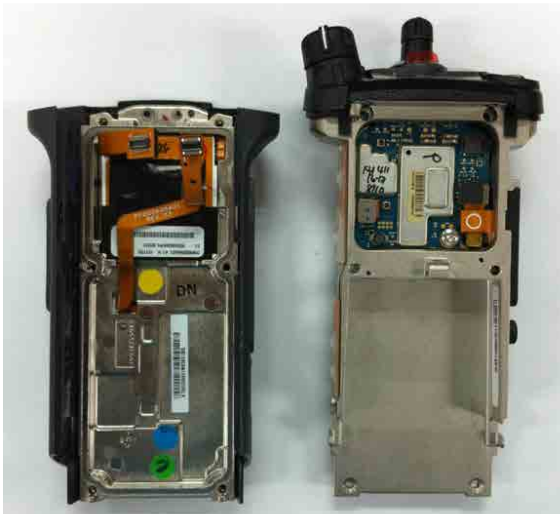
Expansion board with chassis and housing (APX6000/ APX6000Li/APX5000 Model 3.5) (Back side)
