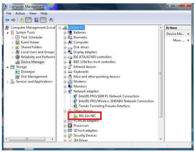
Copy the corresponding driver "MP\_Kit\_RTL11n\_8723BU\_USB\_v28\_20131212" into the PC, and install driver, the installation methods: open the file "MP\_Kit\_RTL11n\_8723BU\_USB\_v28\_20131212", double click "Setup" installation program, guide to install.
