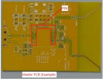
3. Place the Module on the Master PCB. Then solder it in sequence : 1.2.3 This antenna is disable
