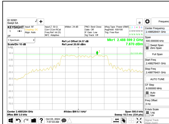
LTE B53 1.4MHz QPSK Middle Channel RB1-0
