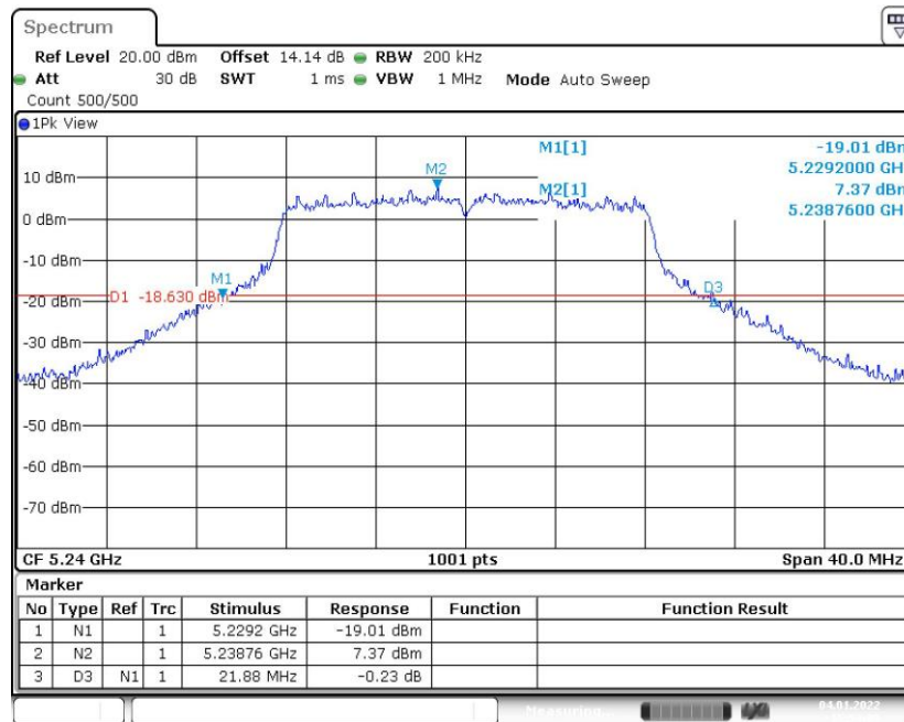
Fig. 3 Occupied 26dB Bandwidth (802.11a, 5240MHz)
