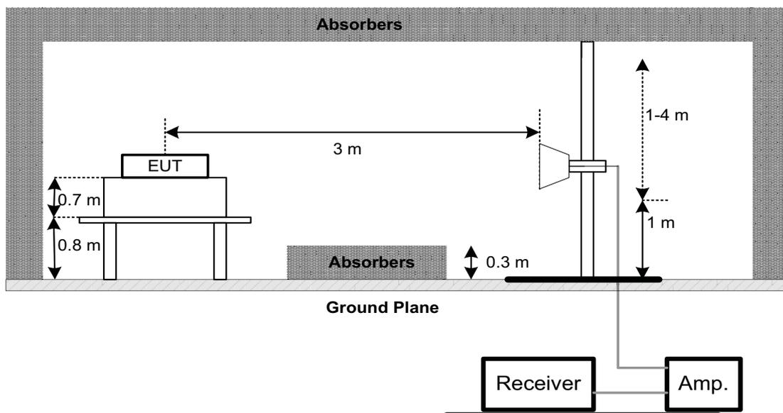
(C) For Radiated Emissions Below 30MHz
