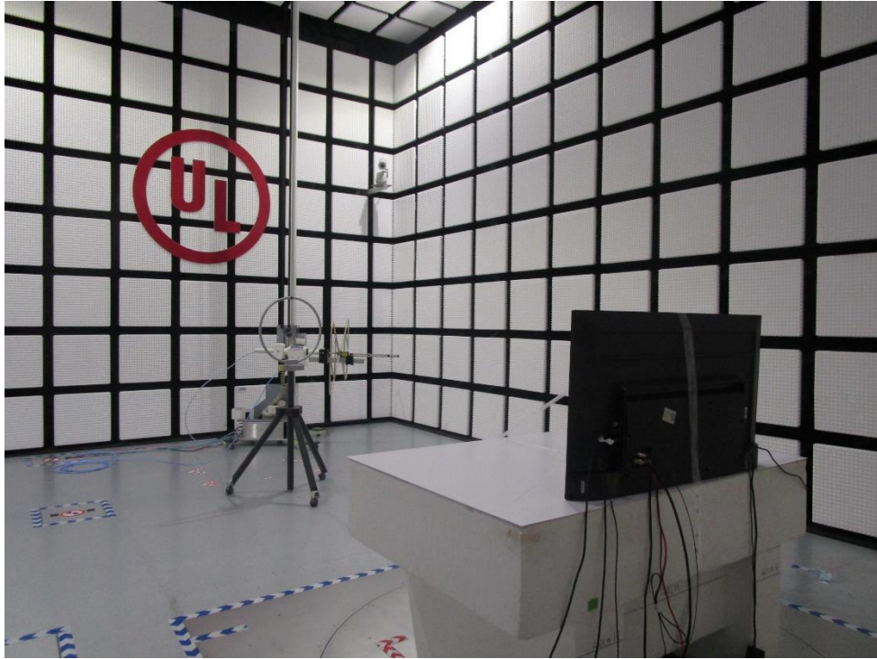
RADIATED RF MEASUREMENT SETUP (Above 1G )
