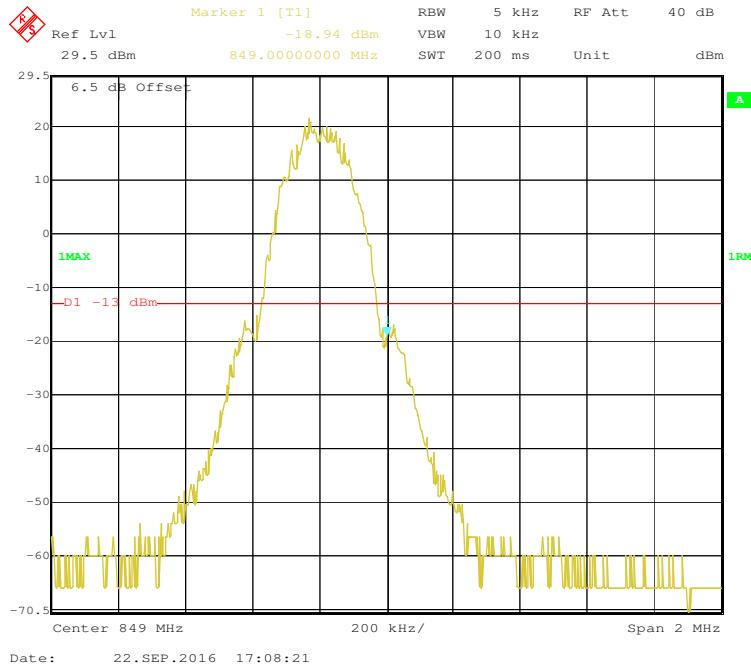
**Cellular Band, Left Band Edge for EGPRS Mode**
