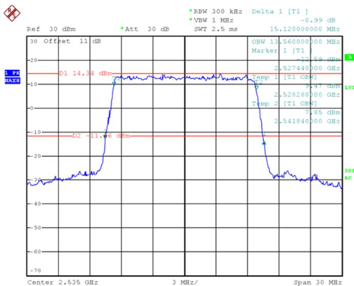
**16-QAM (15.0 MHz) - 99% Occupied & 26 dB Bandwidth, Middle channel**
