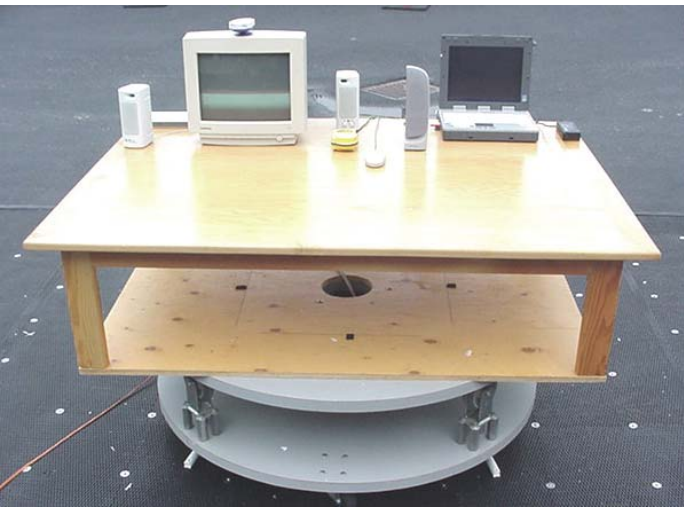
Photograph F-3 - Front of Radiated Emission Configuration
