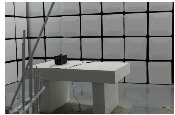
**1.2** Setup for Unwanted Emissions that fall Outside of the Restricted Bands(Radiated) and Unwanted Emissions in the Restricted Bands (Radiated) below 1GHz
