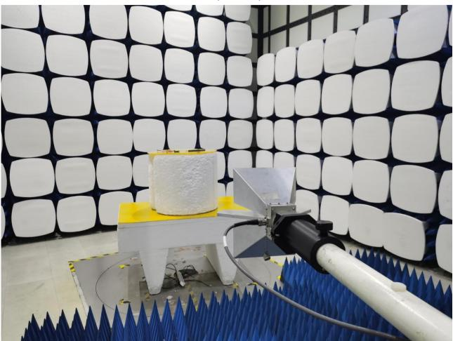
**1.5** Setup for Unwanted Emissions that fall Outside of the Restricted Bands(Radiated) and Unwanted Emissions in the Restricted Bands (Radiated) above 1GHz
