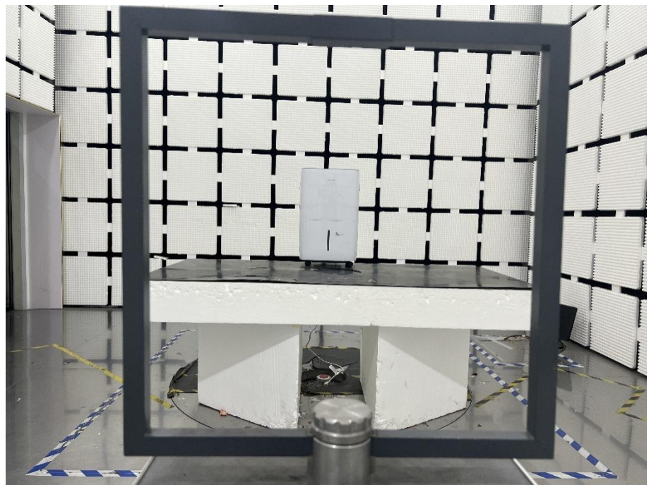
Radiation Emission Test Setup (Below 30MHz)
