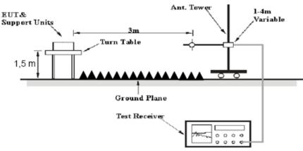
The radiated emission Below 1GHz tests were performed in the 3 meters chamber, above 1GHz tests were performed in the 3 meters chamber B, using the setup accordance with the ANSI C63.10-2013. The specification used was the FCC 15.209, and FCC 15.247 limits.
