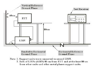
The setup of EUT is according with per ANSI C63.10-2013 measurement procedure. The specification used was with the FCC Part 15.207.
