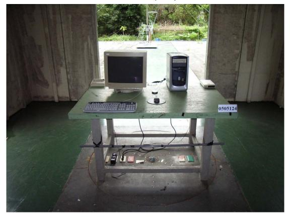
Radiated Emission Test Set-UP, Frequency Between 30 - 1000MHz
