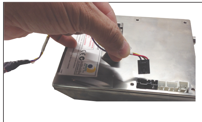
Figure 2. Insert the connector from the power module.
