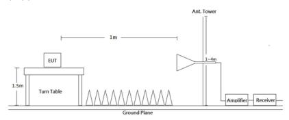
Radiated emission tests were performed in the 3 meters chamber test site, using the setup accordance with the ANSI C63.10-2013. The specification used was the FCC Part 15.209, FCC 15.247 Limits.
