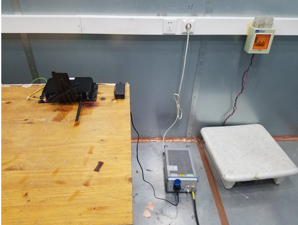
Picture 2 Conducted Emission Test Setup
