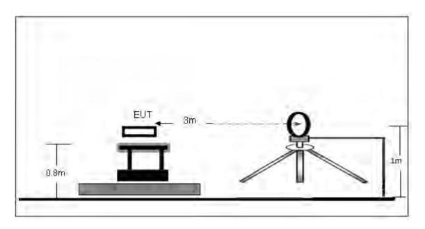
(B) Radiated Emission Test-Up Frequency 30MHz~1GHz
