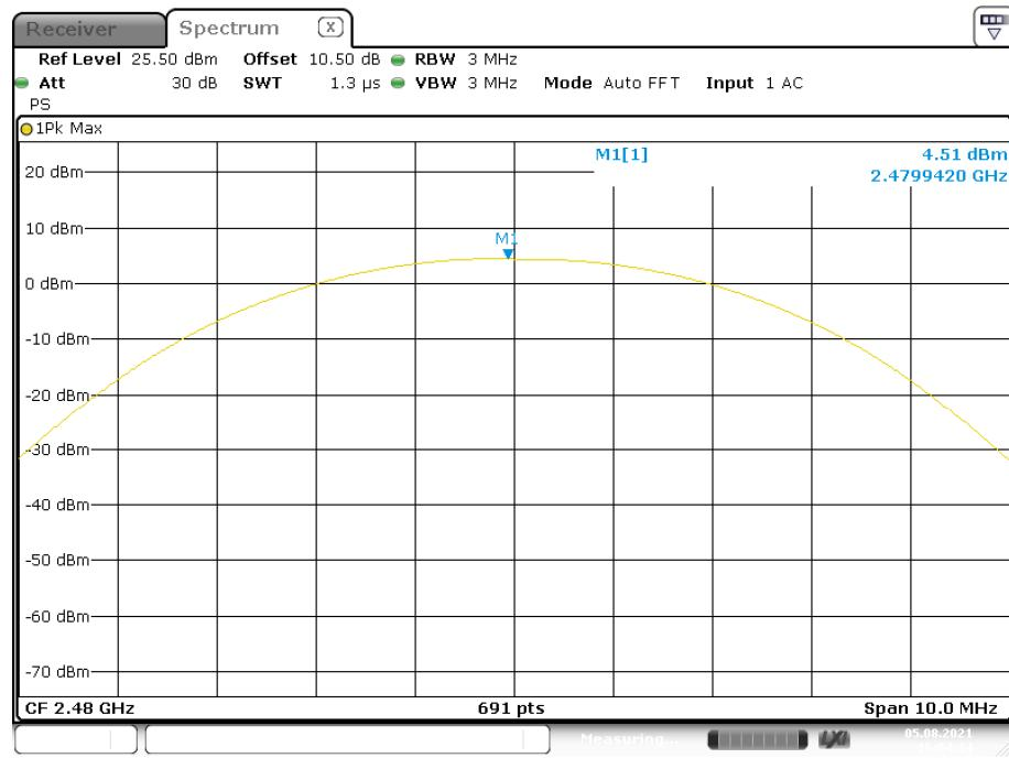
**EDR ( $\pi/4$ -DQPSK): Low Channel**
