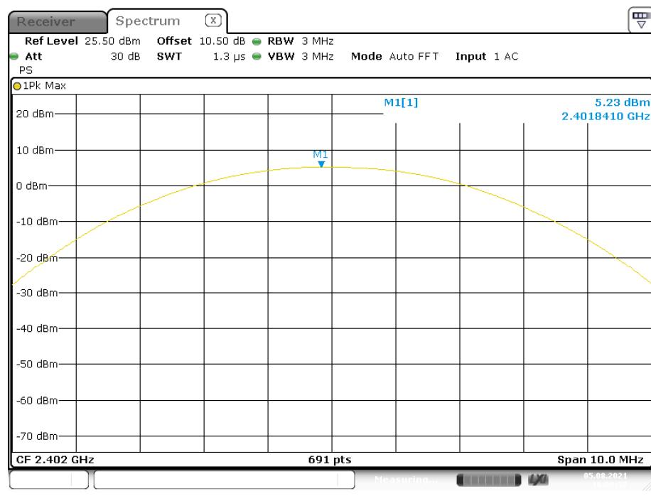
**EDR ( $\pi/4$ -DQPSK): Middle Channel**
