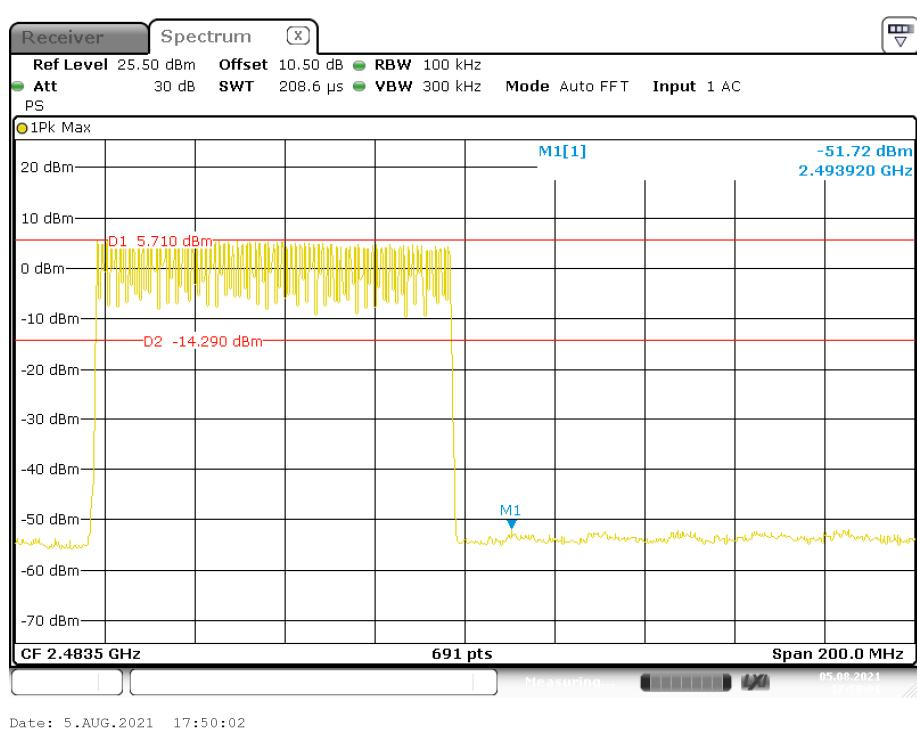
**EDR ( $\pi/4$ -DQPSK): Band Edge-Left Side****Single**
