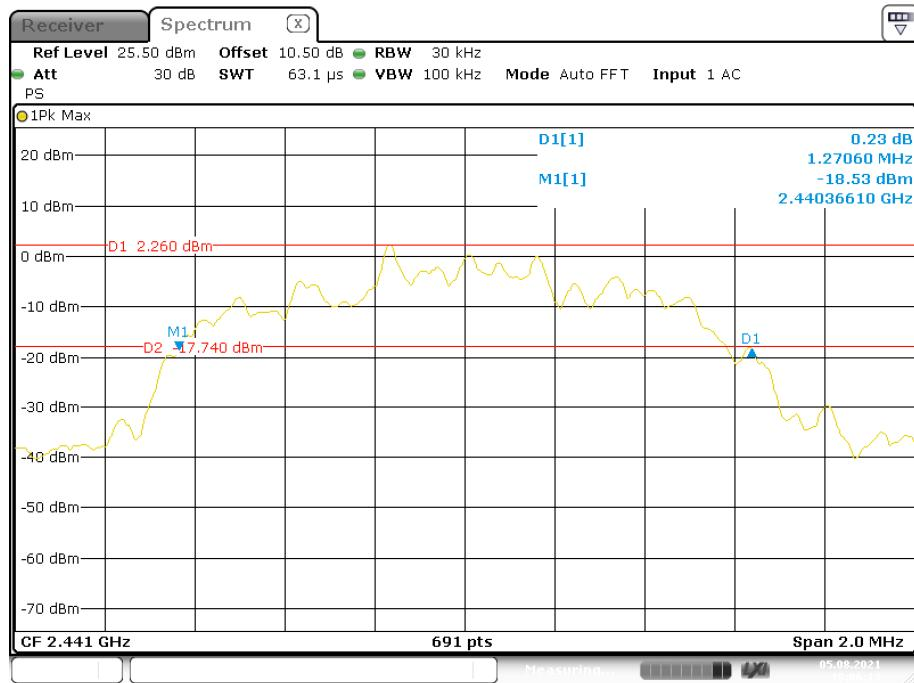
**EDR ( $\pi/4$ -DQPSK): High Channel**
