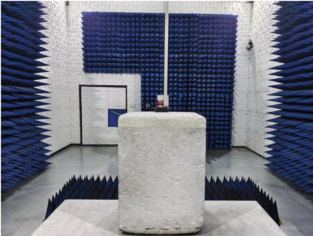
RADIATED EMISSION TEST SETUP ABOVE 1GHZ
